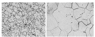
Figure 1: Metallic sample before and after grain growth (from Blikstein & Tschiptschin, 1999)
